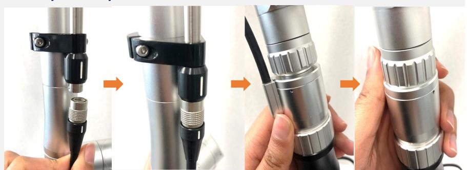
Before replacing the handpiece, make sure the device is turned off. Connect the white part of the handpiece cable to the arm cable and insert. Connect the handpiece to the arm while rotating.
